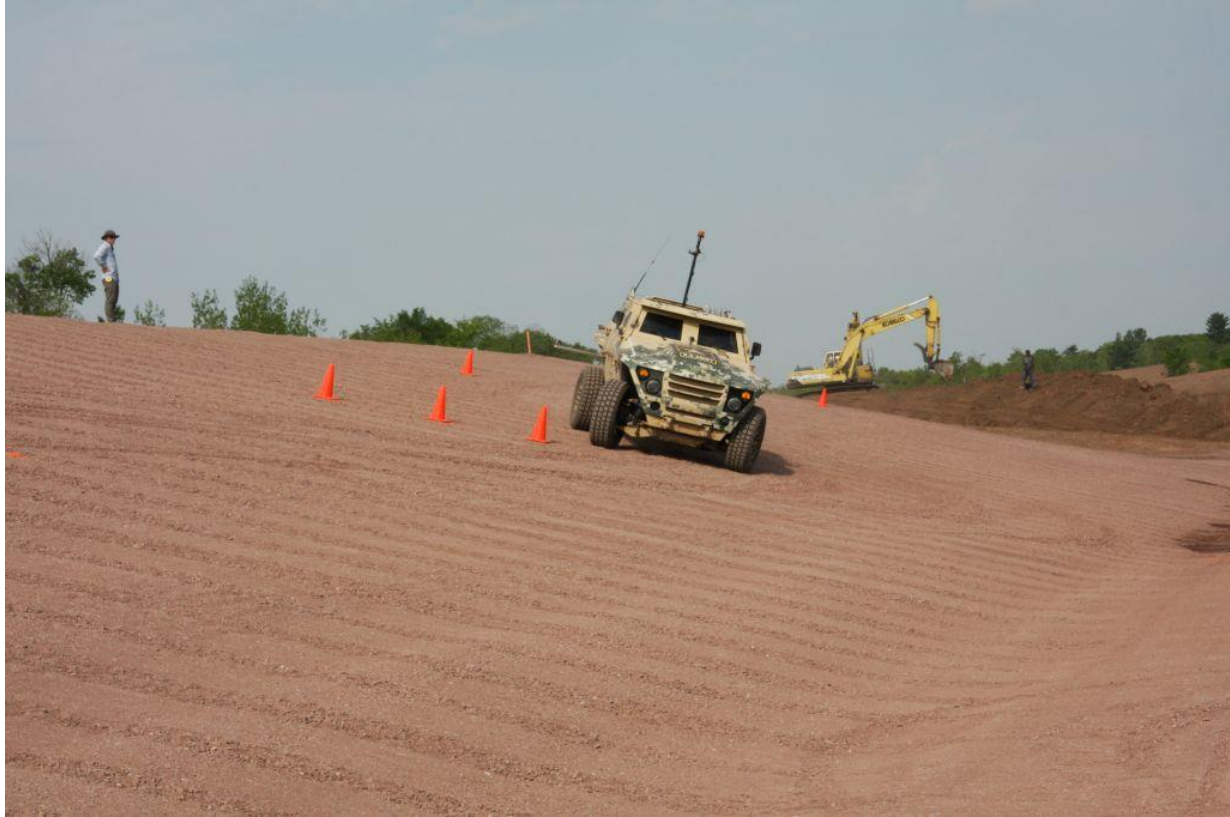
Figure 3.3.1.5-2: FED-A navigating side slope
