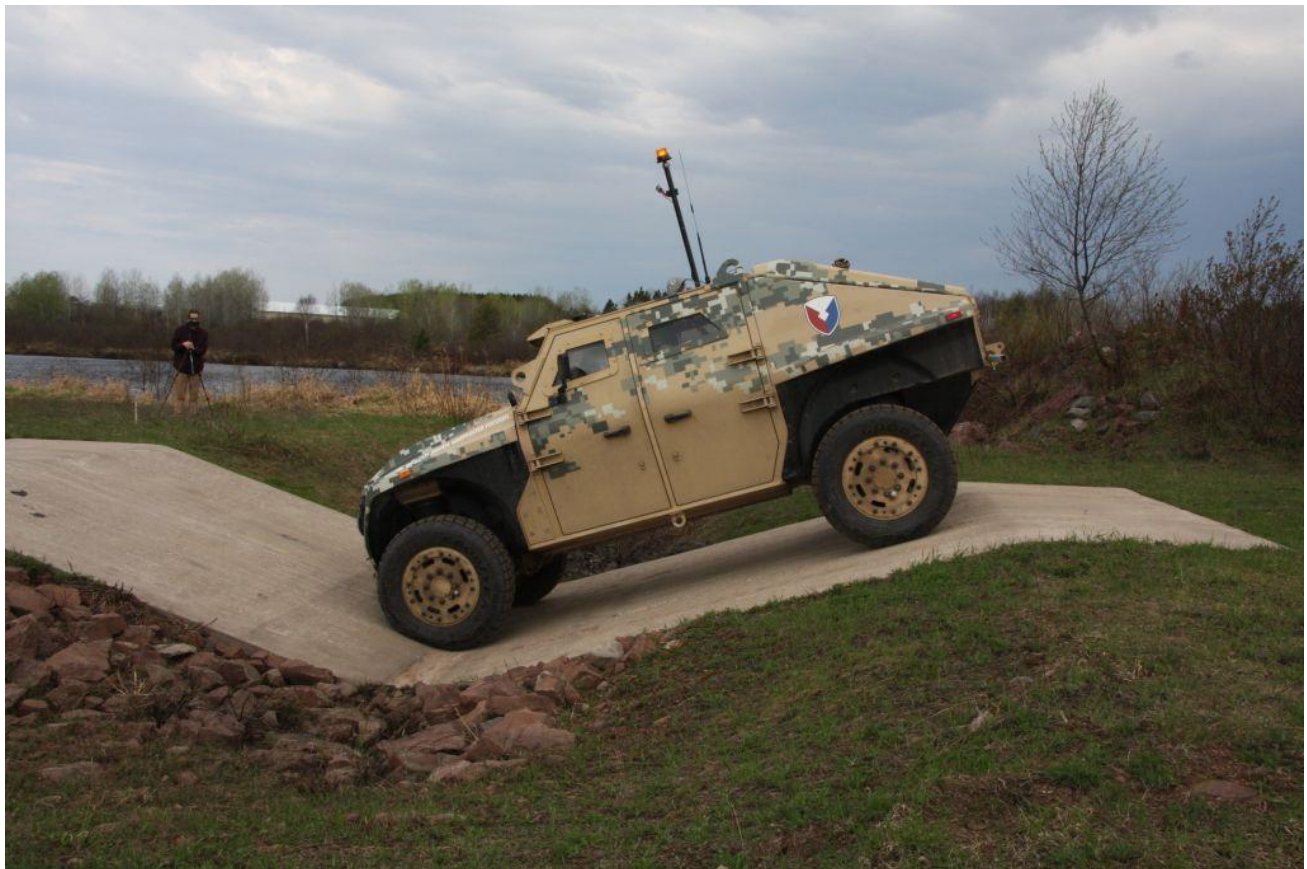
Figure 3.3.3.1-1: Vehicle crossing a 35% V-ditch with 25.5 foot span
