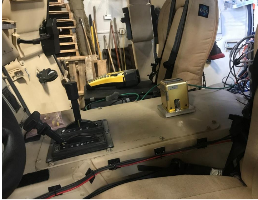
Figure 3.2.3-2: Installation of the MotionPak, Near the Vehicle COG
