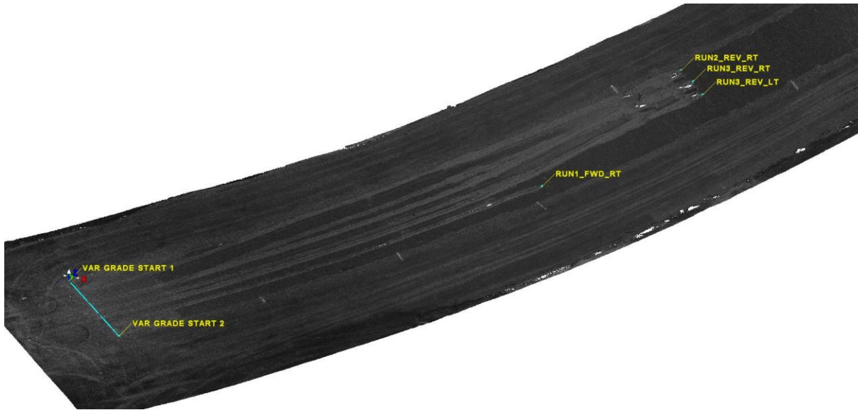
Figure 3.4.1-3: Terrestrial LIDAR Scan of the Wheel Ruts Made During Sand Slope Testing
