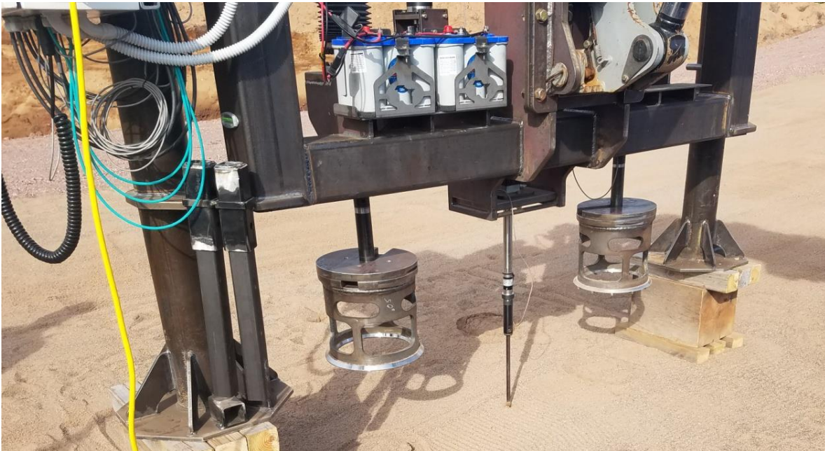
Figure 2.2.3.2-1 KRC Bevameter with Cone Penetrometer Shown in Pressure Sinkage Actuator Location
