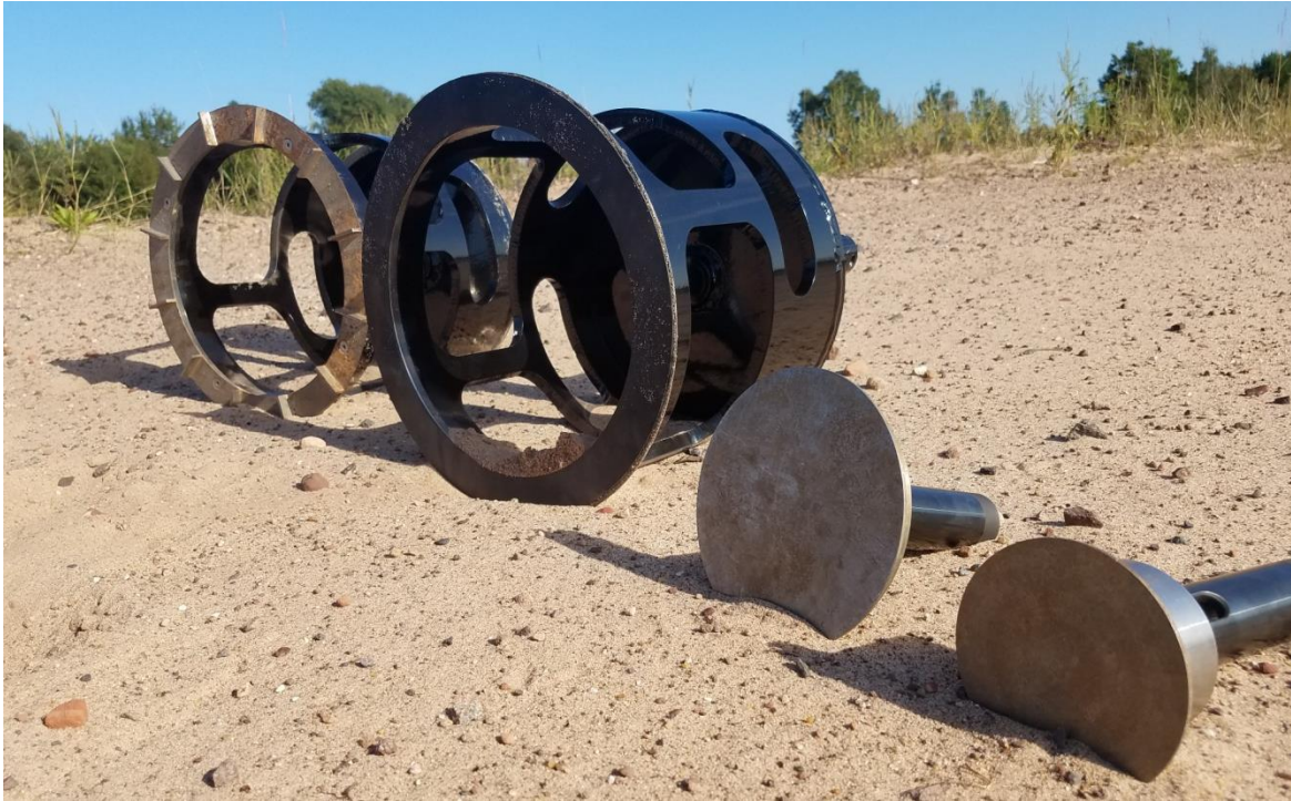
Figure 2.2.3.2-2 The Four Bevameter Measurement Heads Used During the CDT
