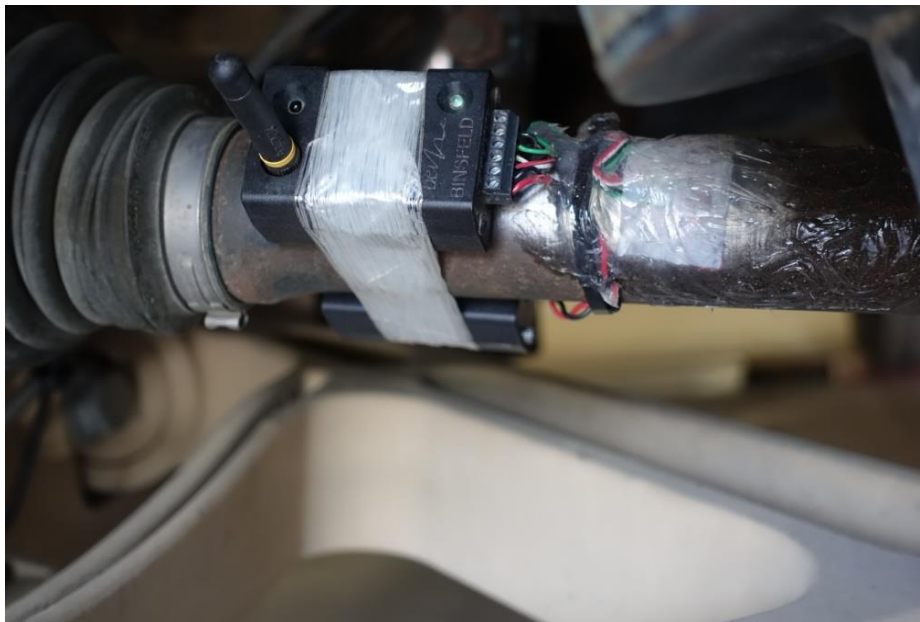
Figure 3.2.10-1: Instrumented Half-Shaft with Binsfeld TorqueTrak Telemetry Transmitter
