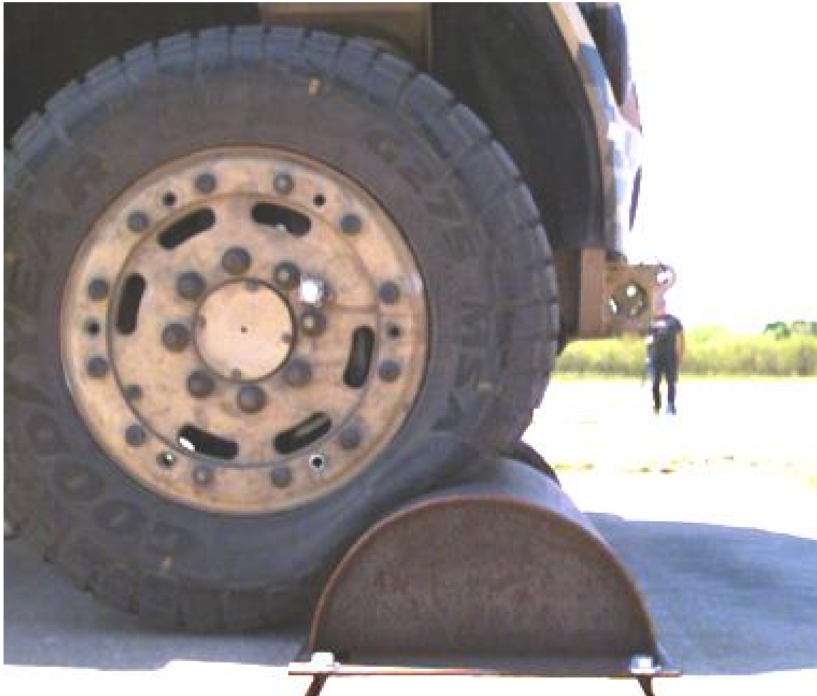
Figure 3.3.2.1-3: Tire deformation over half-round (High Speed Video of All Runs Is Available)
