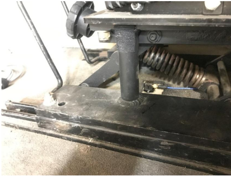
Figure 3.2.4-2: Seat Base Accelerometer (Driver's Side)
