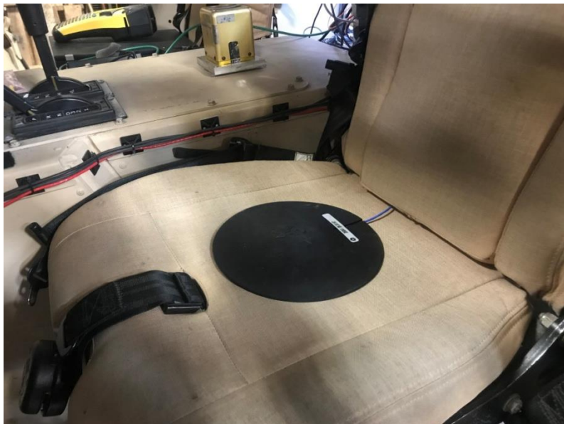
Figure 3.2.4-1: Seat Pad Accelerometer (Driver's Side)
