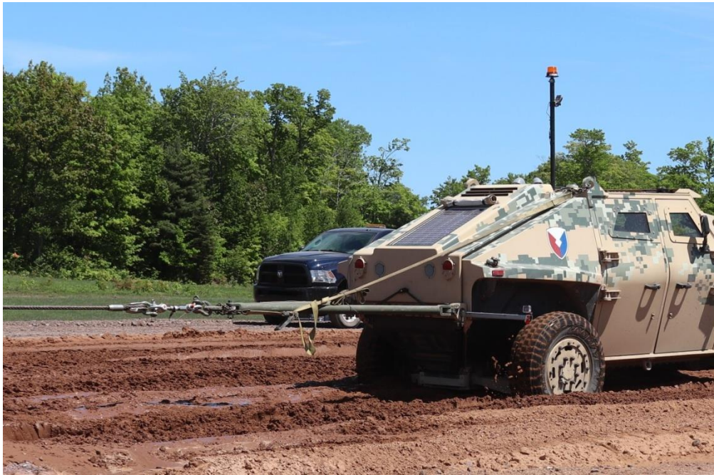
Figure 3.2.11-2: Drawbar and Loadcell Installed on FED-A
